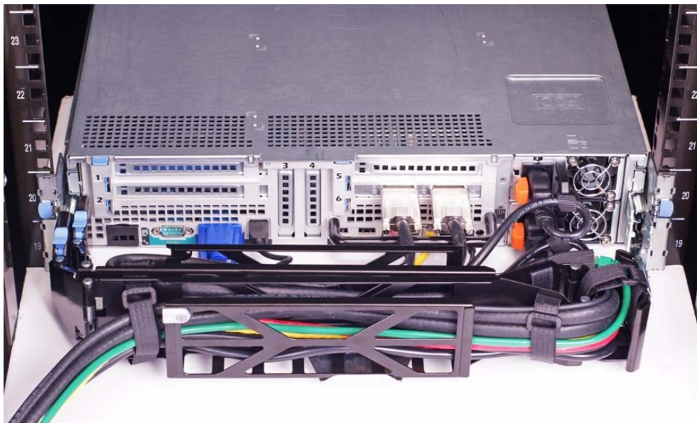
Figure 4: Left-Side Mounted CMA Installation
