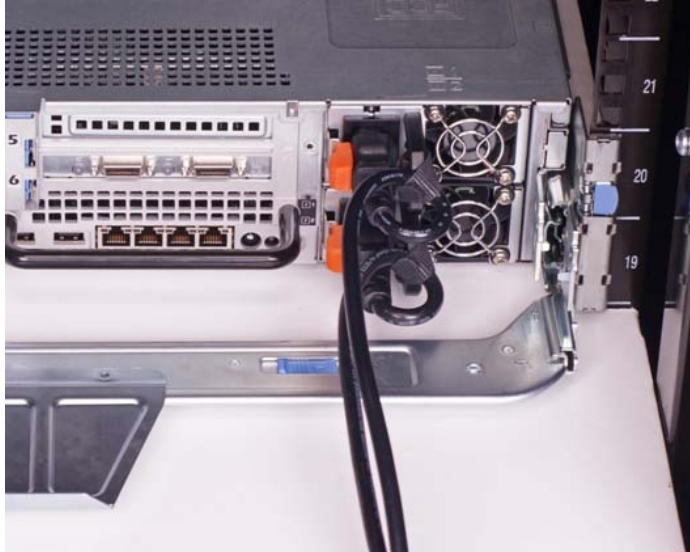
Figure 2: Routing Power Cables Through the Strain Reliefs
